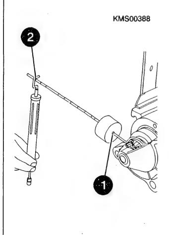
Checking overrunning clutch torque
